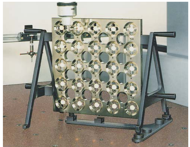
Fig. 3: KOBA-check sphere plate in vertical position with adaptor plate and additional lateral support
